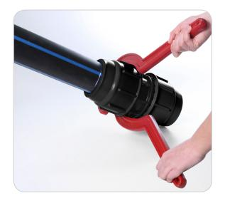
The nut should be screwed tightly, however there is no need for the nut to actually meet the body shoulder.
